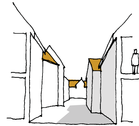
Width of space equal to or less than height of enclosing planes
