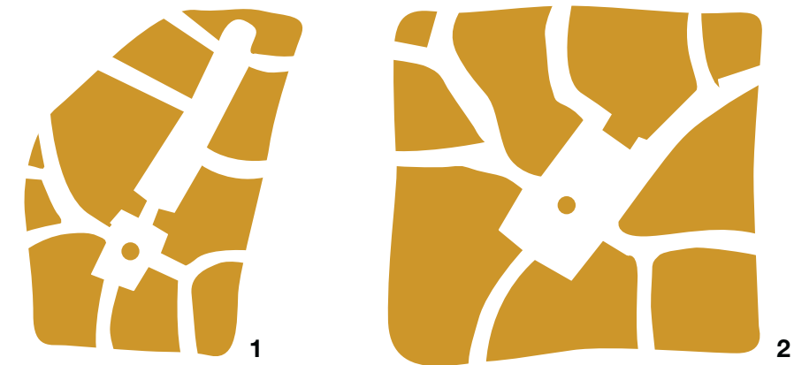
1. Dynamic formal space – length should be limited to avoid monotony for the pedestrian 2. Static formal space in matrix of informal layout
