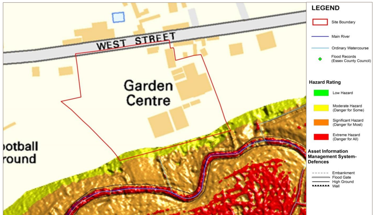
Figure D River Blackwater flood hazard mapping for the site - 0.1% AEP scenario (proxy for 1% plus 35% climate change)
