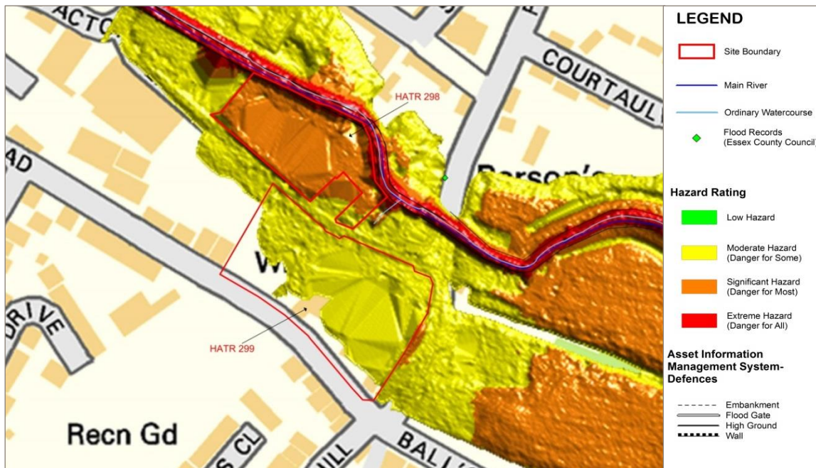
Figure E River Colne flood Hazard modelling for the site - defended 1% AEP including an allowance for climate change
