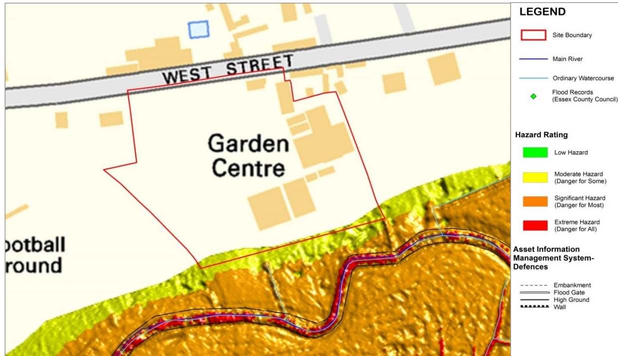
Figure D River Blackwater flood hazard mapping for the site - 0.1% AEP scenario (proxy for 1% plus 35% climate change)
