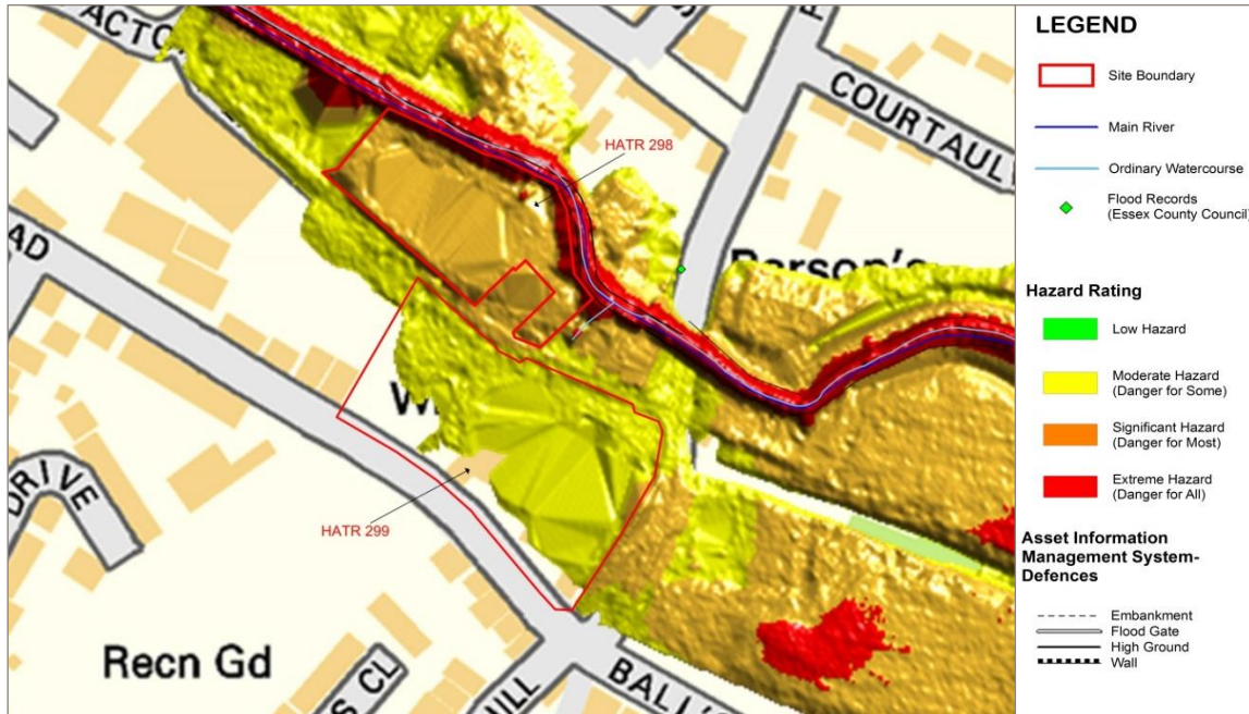
Figure D River Colne flood Hazard modelling for the site - undefended 1% AEP including an allowance for climate change
